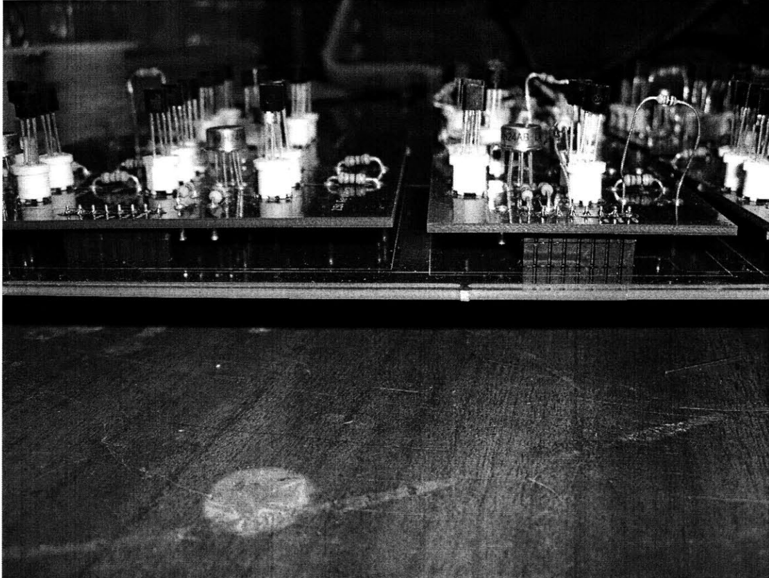
Figure 5-3. Side view of laboratory kit. Individual modules plug in to main board via SIP connector with 0.1" spacing for breadboard compatibility.
