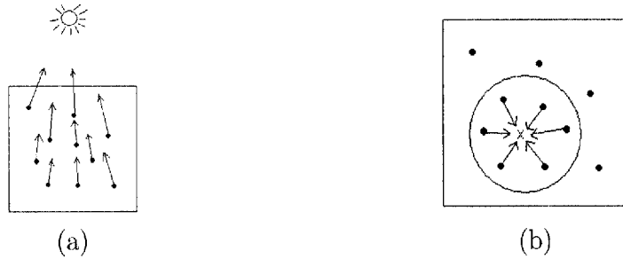
Figure 3-4: Before rendering, the irradiance is sampled and cached at many points covering the surface of the skin (a). When a point is being shaded, the contributions of all of the points within range are summed (b).
