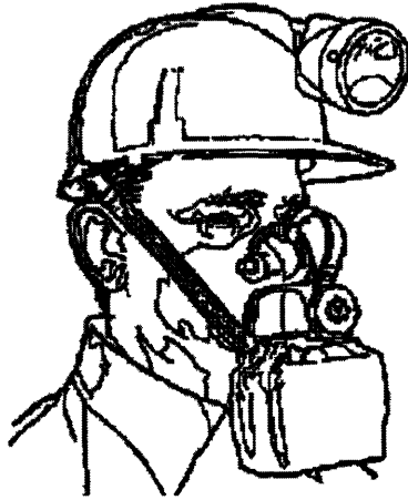
Figure 5: Mine Safety Appliances Company Model W-65 filter self-rescue device shown being worn by a miner. The device clips the nose shut and delivers filtered air to the mouth. 13
