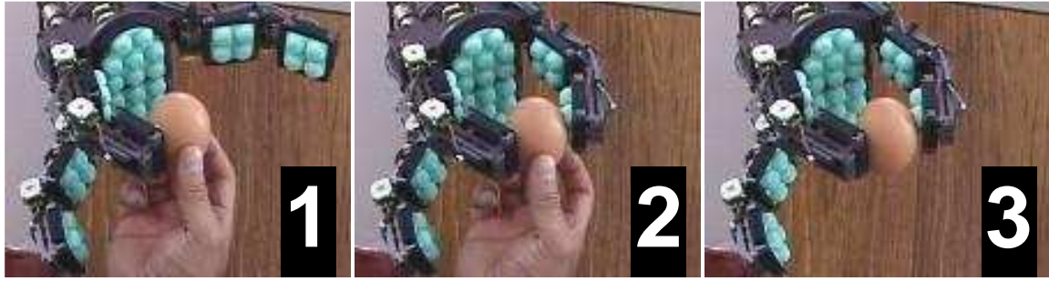
Figure 5-8: In this sequence we observe the hand closing on a egg. This task is easier than the one shown in figure 5-9. If we observe carefully 3. we can notice the properties of the tactile sensors. They detect the contact but also conform to the object increasing friction and making an stable grasp possible.
