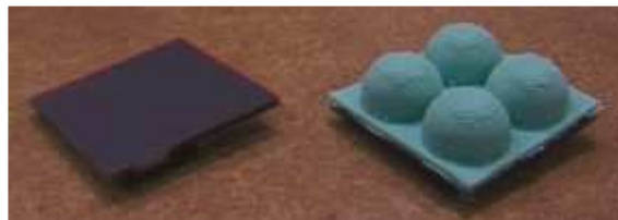
Figure 2-19: Left: A commercial FSR tactile sensor with high spatial resolution (200 point per square inch), flat surface, rigid, and low friction coefficient. Right: OBRERO's tactile sensor with low spatial resolution (about 16 points per square inch), dome-like surface, flexible, and higher friction coefficient.
