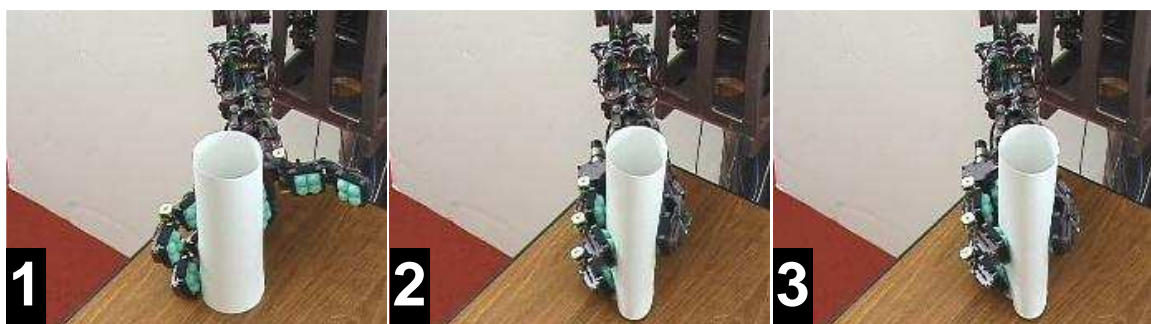
Figure 5-10: In this sequence the robot closes its fingers without using tactile feedback. As a consequence they crush the object.
