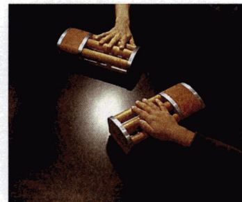
Figure 4: Two users communicate force and motion through their respective inTouch device [08].
