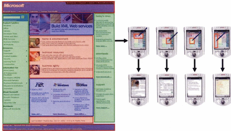
Figure 2-9: The FOM approach attempts to categorize graphical objects by their function. The navigational column in this graphic is recognized as such and can be rendered according to navigational needs. This also allows interaction adjustments. For instance, the navigational elements might produce a menu when the users clicks in that region.
