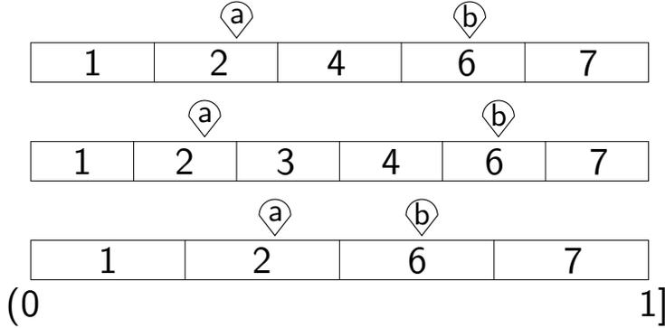
Figure 4.7: Fixing the threat label parameter. Markers **a** and **b** represent two floating-point numbers on the interval  $(0, 1]$  which represent threats 2 and 6, respectively. The UAV discovers threat 3 between the top line and the second, and then the UAV disables threats 3 and 4 between the second and the third. In each case, the numbers **a** and **b** must be scaled to stay in the same position relative to the threats they represent.
