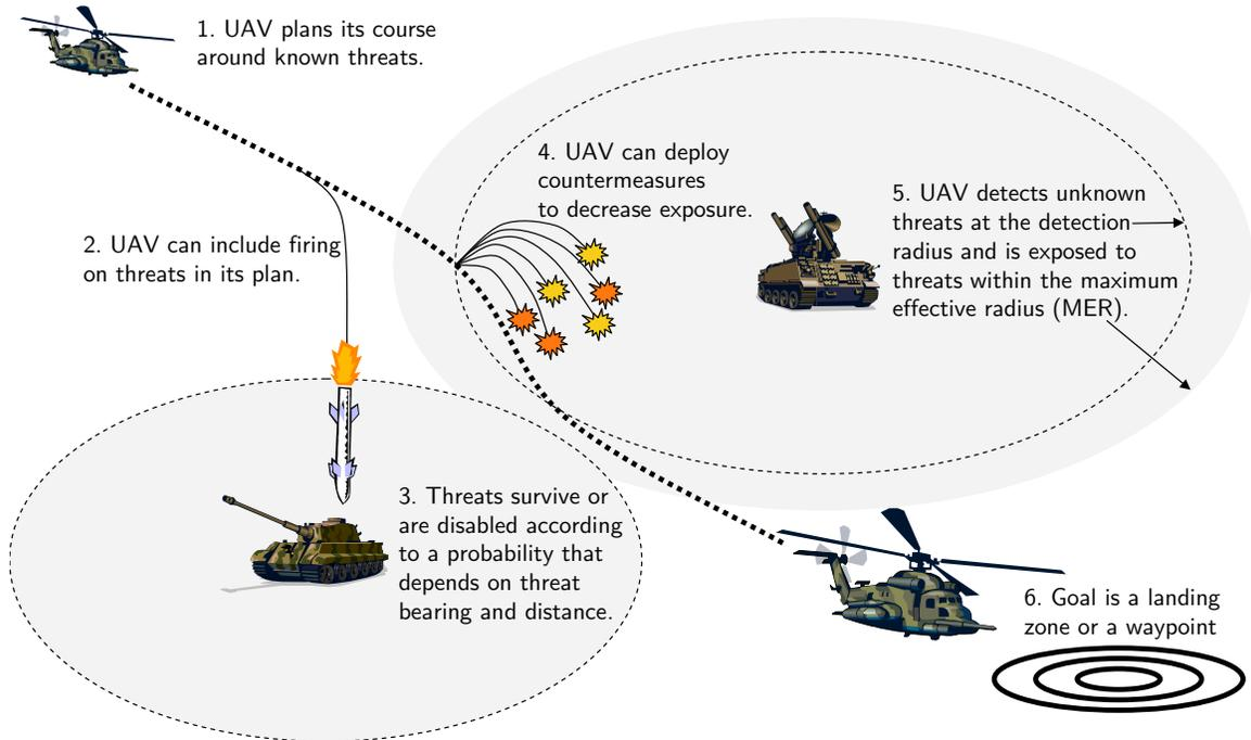
Figure 4.1: In the threats problem, the UAV navigates to reach the goal quickly while minimizing exposure to threats. It also can fire on threats and deploy countermeasures.
