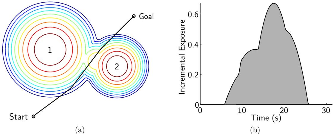
Figure 4.2: Exposure calculation for a trajectory through two adjacent threat regions. The black line represents the vehicle trajectory. As the UAV traverses the threat regions (a), it accumulates exposure. The total exposure is the integral of the incremental exposure, and is therefore equal to the area in grey (b).
