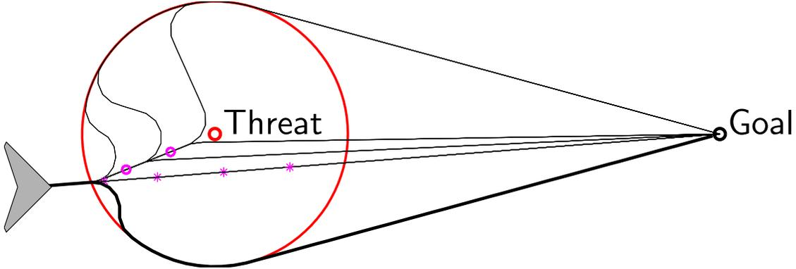
Figure 4.8: Candidate reactive plans. The plan with the highest fitness is shown in bold. Magenta circles denote positions from which the UAV fires, and magenta stars denote countermeasures.
