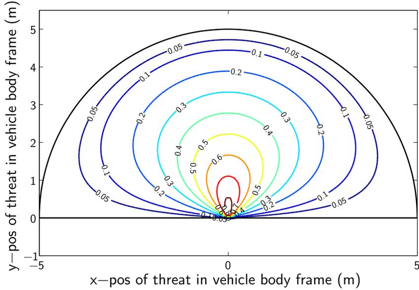
Figure 4.3: Probability of disabling a threat. Distance and bearing determine the probability function, but here contours are shown in Cartesian coordinates. The positive  $y$  axis corresponds to the UAV’s forward direction.
