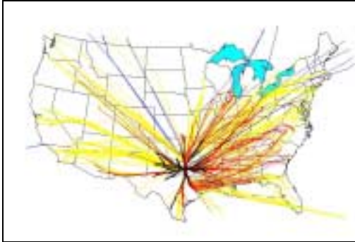
Figure 20: Trajectories for DFW Departing Flights (turboprops in black, regional jets in red, narrow body jets in yellow, wide body jets in blue)
