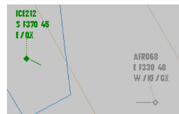
Figure 10: Aircraft icons from the University of Iceland prototype show secondary radar data (right) and secondary data reinforced with primary radar data (left).
