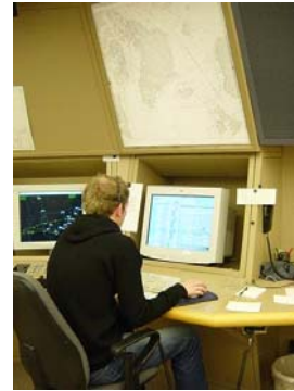
Figure 5: The Reykjavik controller workstation consists of electronic flight strips, in front of the controller and a situation display, to the left of the controller.
