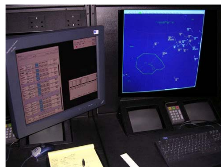
Figure 11: Advanced Technologies and Oceanic Procedures (ATOP) is the future Oceanic workstation for the United States. Implementation at Oakland, Anchorage, and New York Center will begin in year 2004.
