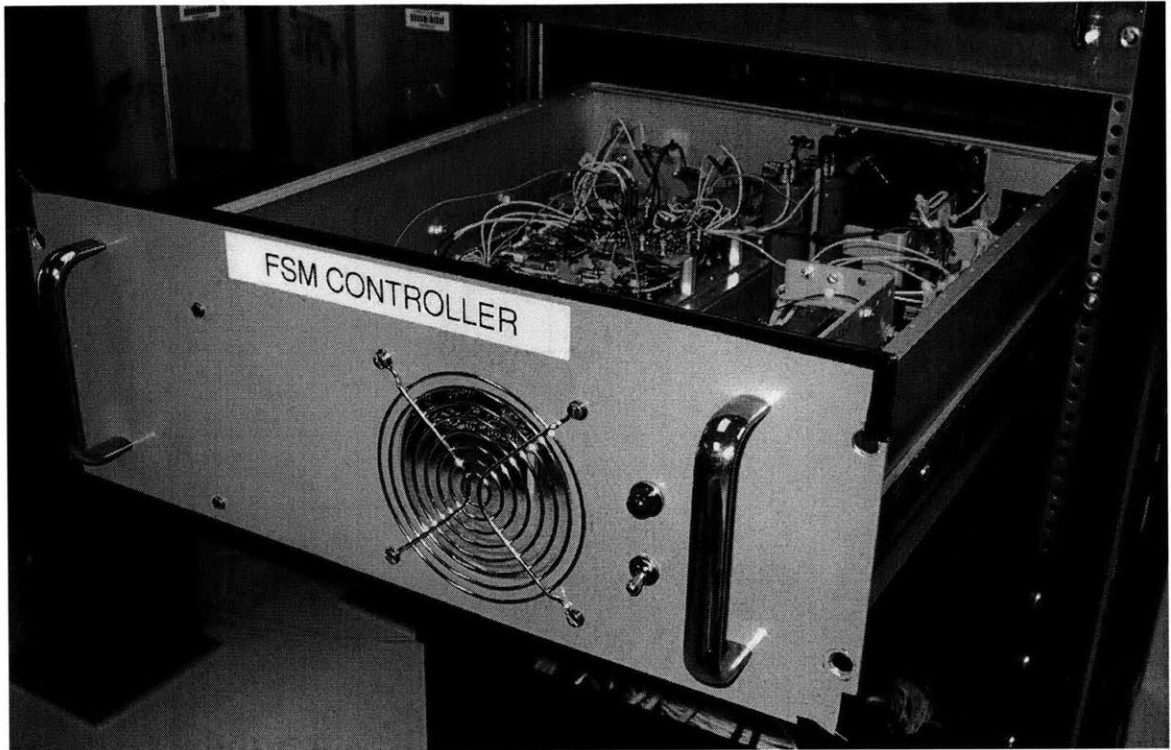
Figure 2-15: Picture of the original controller hardware box mounted in rack, housing the analog compensator, current amplifiers and power supplies.
