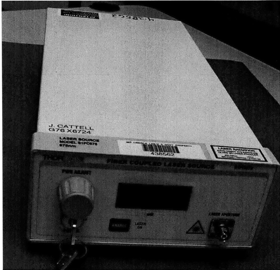
Figure 2-2: Picture of the Thorlabs fiber-coupled laser source, model S1FC675.
