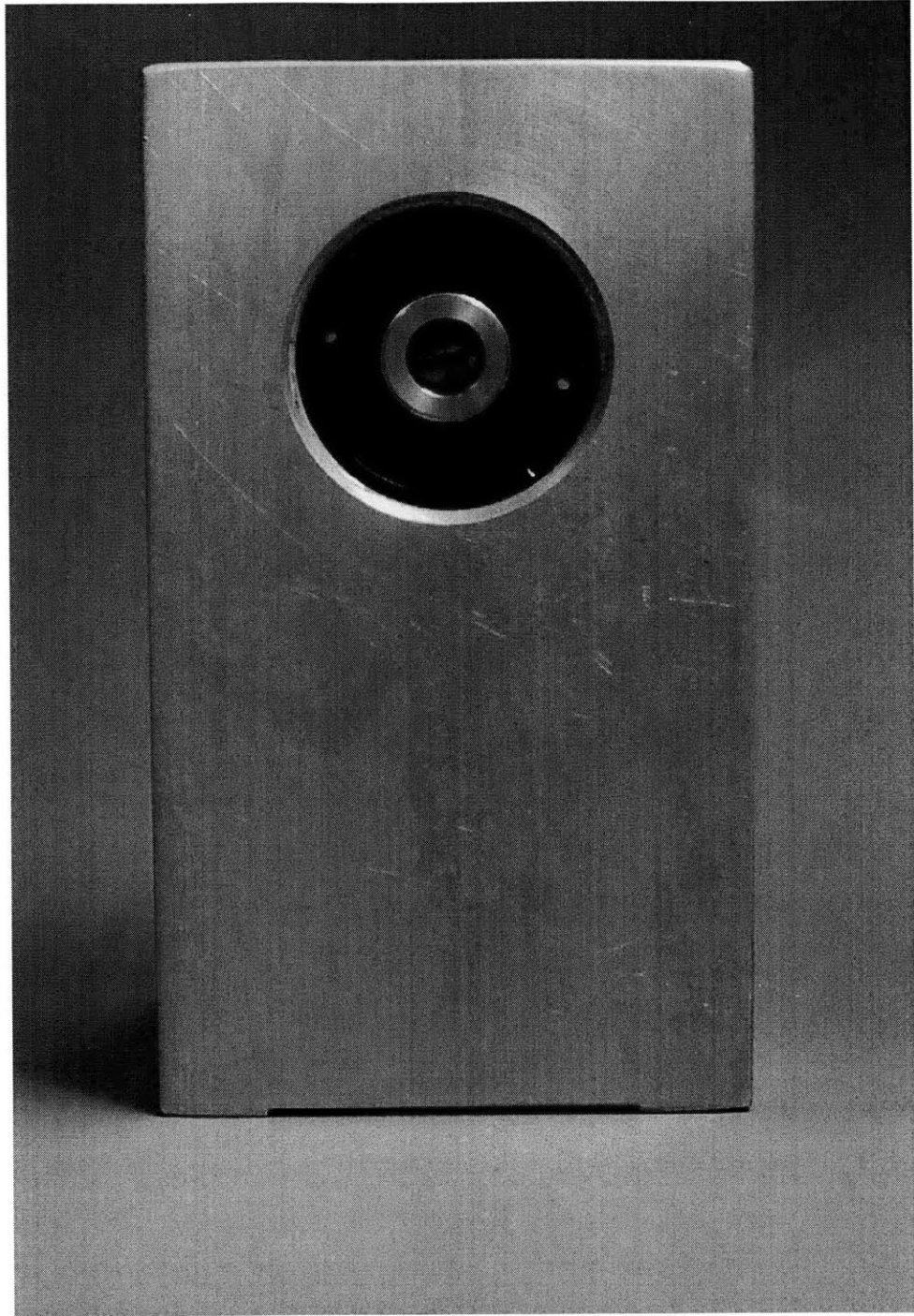
Figure 2-3: Picture of the collimator used with the fiber-coupled laser source in mount, courtesy of Paula Ward.
