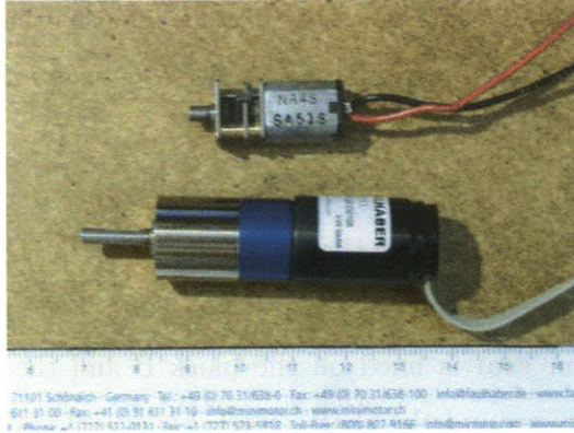
Figure 3-13: The motors used for the Shady3D robot. The upper is a Sanyo NA4S mini gearmotor with a 298:1 gearhead. This is used for the gripper opening/closing mechanism. The lower is a MocoMo 1724T006SR DC micromotor combined with a 66:1 gearhead. This is used for joint actuation.
