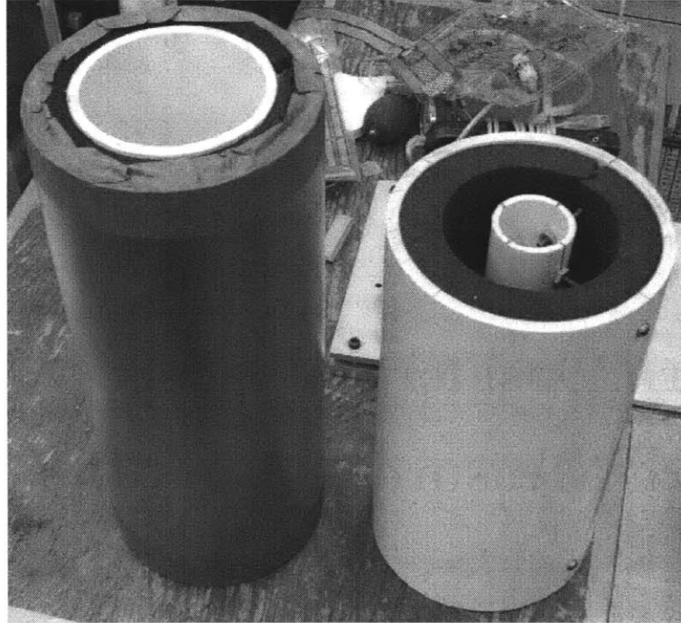
Figure A-1: Soft cylindrical test rigs: (left) test rig intended for use in the elastic bindings tests; (right) calibration rig.
