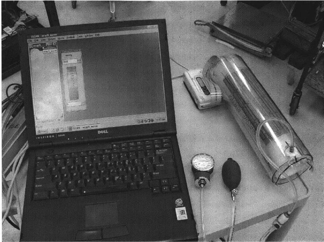
Figure 3-2: Tekscan I-Scan system undergoing calibration in the cylindrical calibration rig, consisting of two concentric rigid cylinders separated by a 10mm channel (right). A known load is being applied to the sensors by inflating a plastic bag inside the channel to a known pressure using the black hand pump (center), as measured by the rotary pressure gage (center). The pressure distribution being measured by the sensors is recorded and displayed graphically on the computer screen (left).
