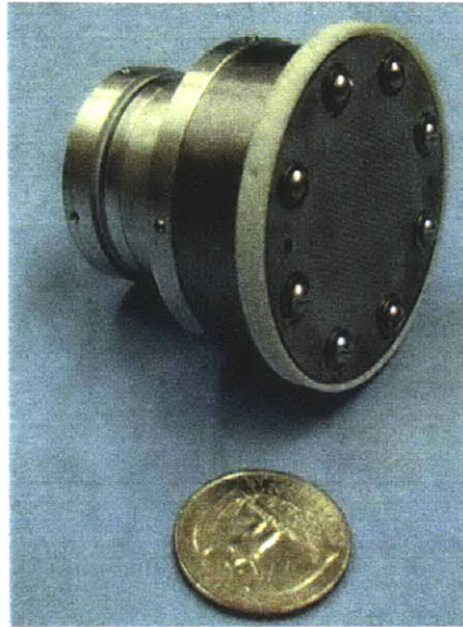
Figure 37: MiXI 3cm ion thruster by JPL [23].
