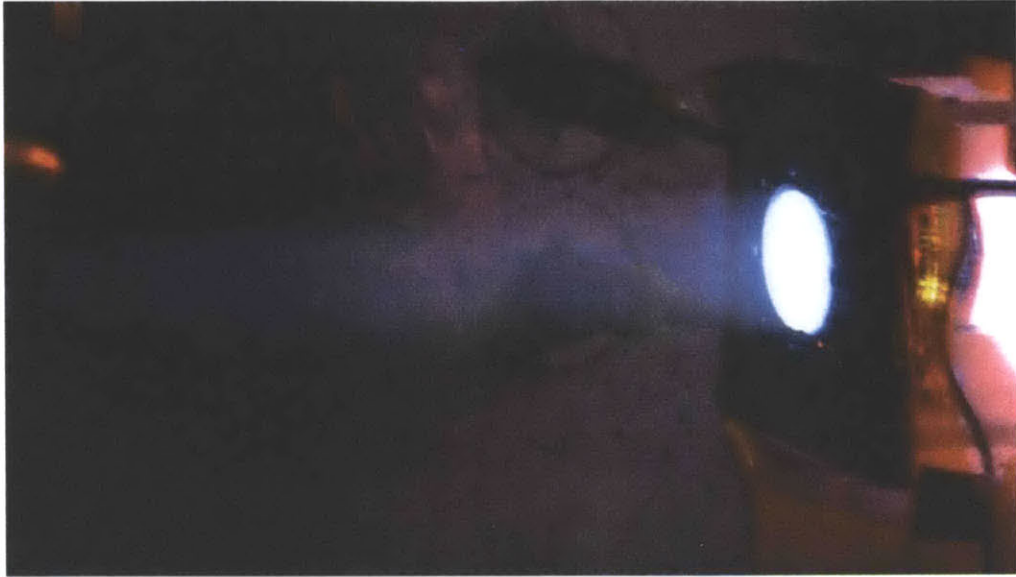
Figure 3: RF micro ion thruster operating in a vacuum chamber.
