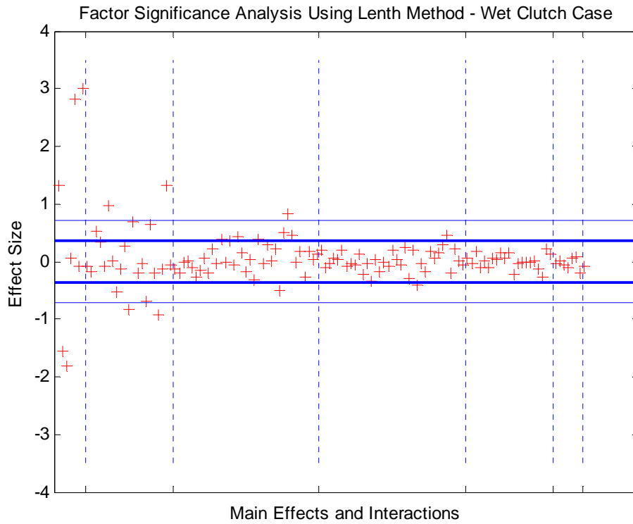
Figure 12 Effect analysis using the Lenth method for the wet-clutch experiment
