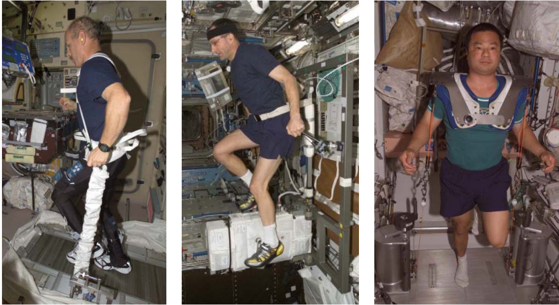
Figure 1.2. Exercise facilities available on the ISS including (a) Treadmill with a Vibration Isolation and Stabilization System, (b) Cycle Ergometer with Vibration Isolation and Stabilization System, (c) Interim Resistive Exercise Device. (reproduced from [12], NASA photography)
