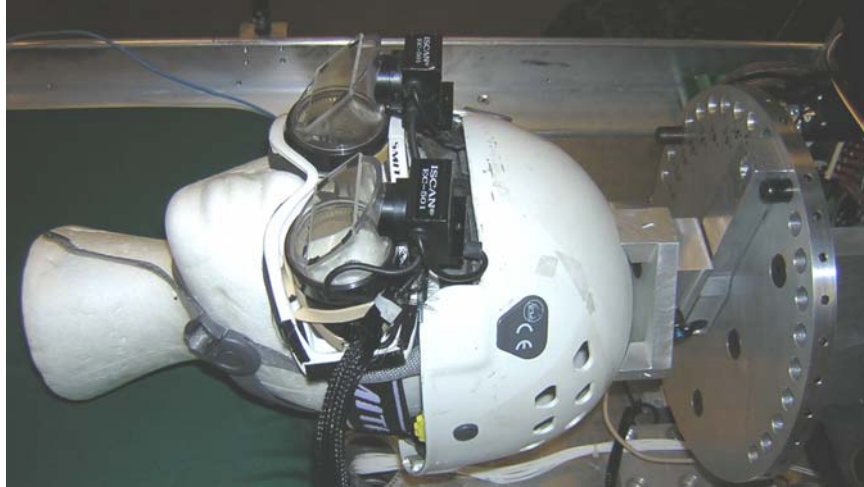
Figure 3.7. ISCAN ® eye tracking system mounted into a ski mask. The helmet and the device to constrain the head-turns into the yaw plane are shown.
