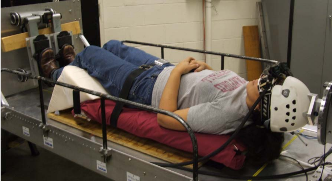
Figure 3.4. Subject lying on the Man-Vehicle Laboratory short-radius centrifuge at MIT (credits: Paul Elias).
