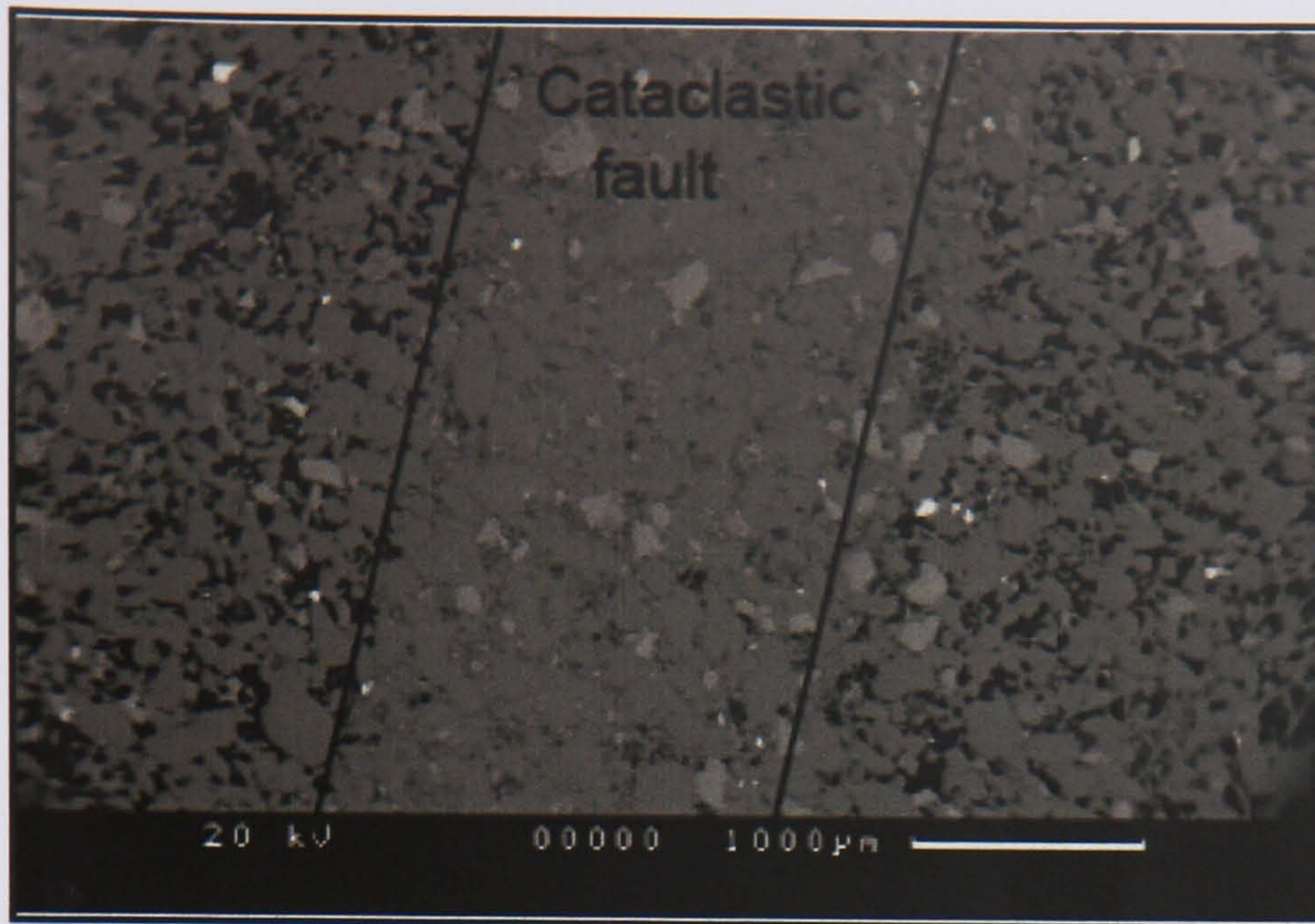
Fig. 4.20. BSE micrograph showing the undeformed sandstone and the cataclastic fault in sample 23/27-8.4, Pierce Field.
