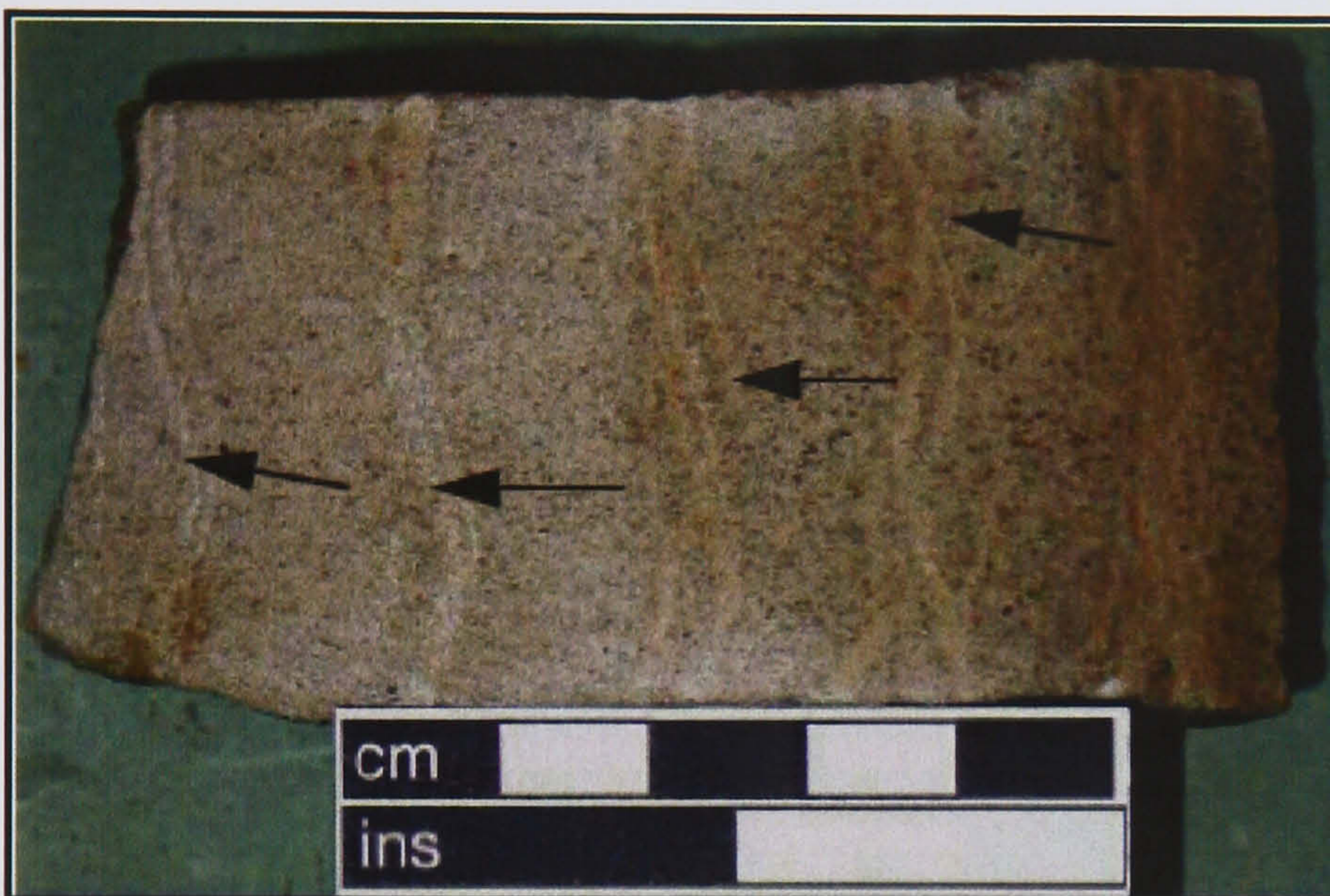
Fig. 4.22. Core photo showing the calcite-cemented fractures (arrows) in sample 23/27-8.7 (depth 8322')
