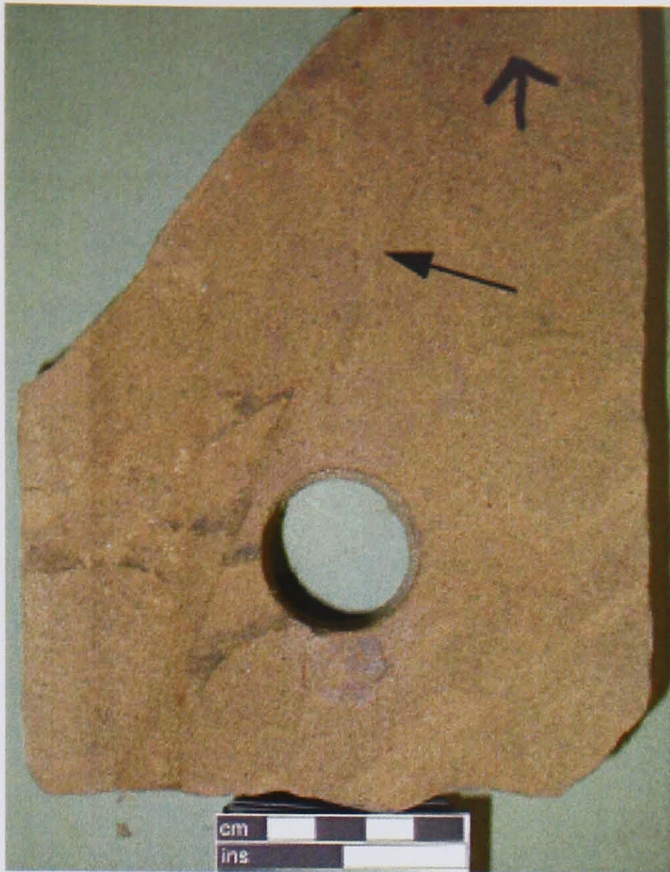
Fig. A.1. Photograph of the hand specimen of sample 23/27-8.1. Note that it contains a thin cataclastic fault (arrow).
