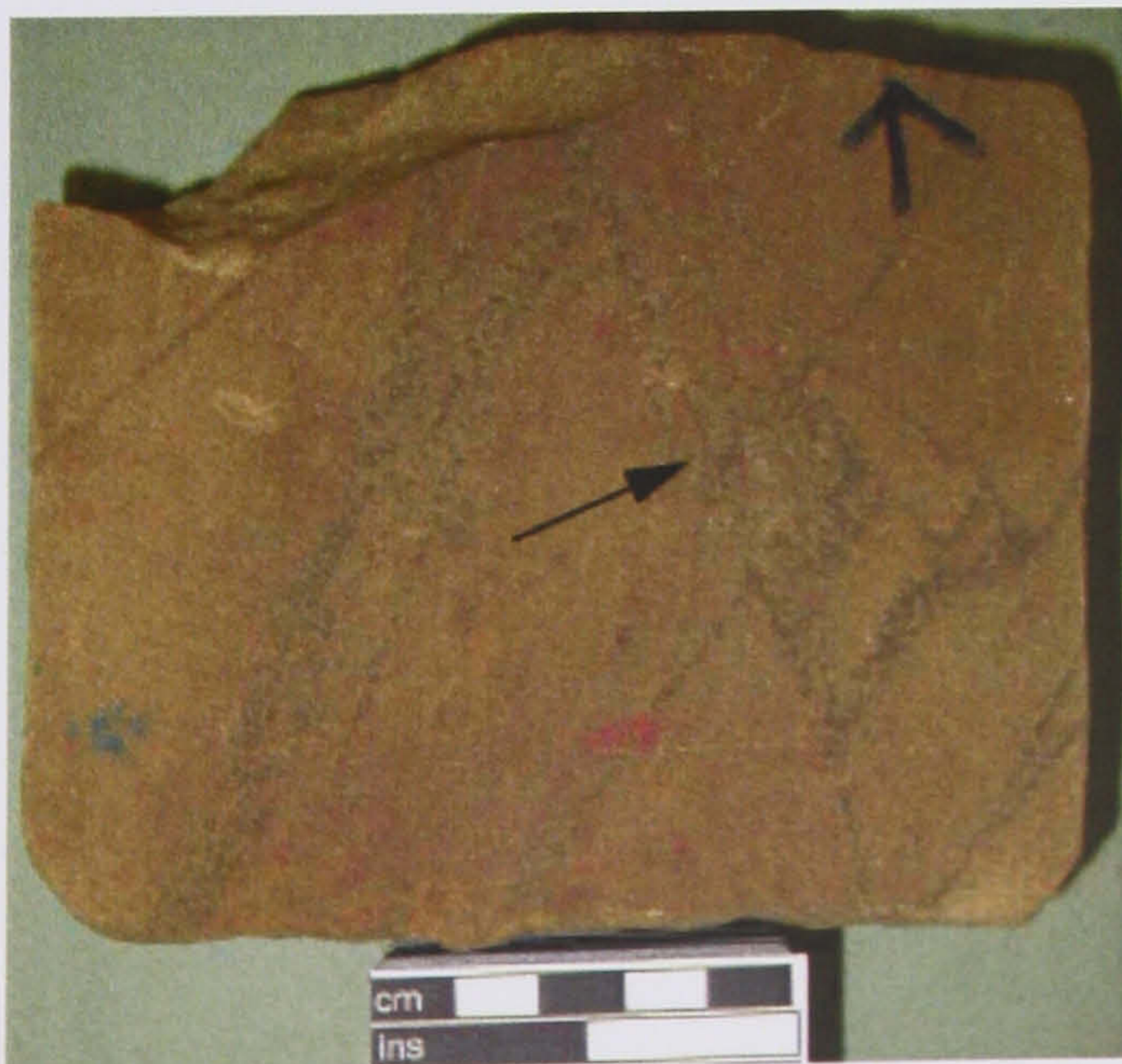
Fig. A.7. Photograph of the hand specimen of sample 23/27-8.3. Note that it contains a thin cataclastic fault (arrow).
