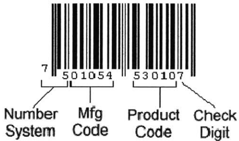
Figure 5: A typical EAN-13 barcode xxxiii
