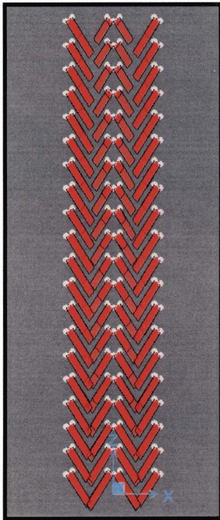
Figure 41. Axial forces on diagonals under dead loads
