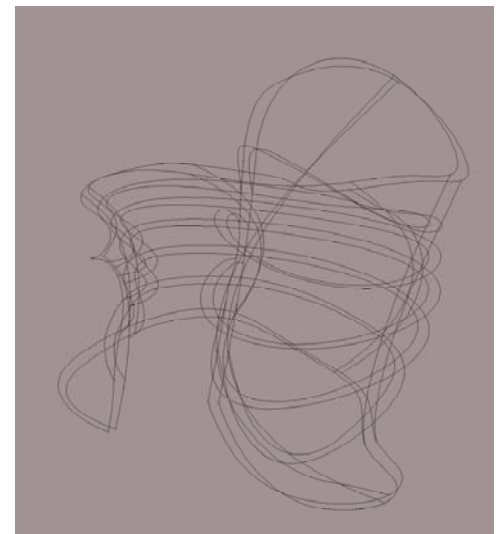
Figure 3.34 Creation of grid Isocurves are extracted from the form for creating a grid that defines each unit
