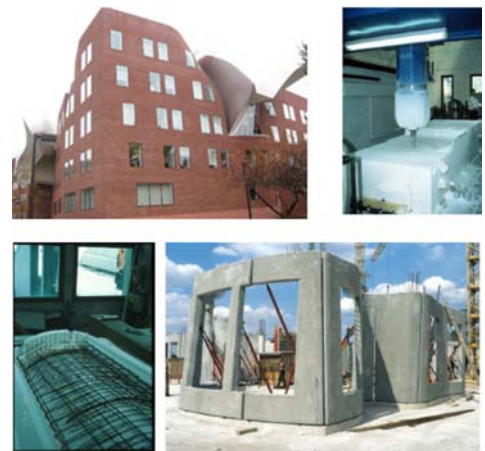
Figure 1.1 Fabrication of Styrofoam molds PROJECT: Case Western Reserve University LOCATION: Cleveland, Ohio ARCHITECT: Gehry Partners
