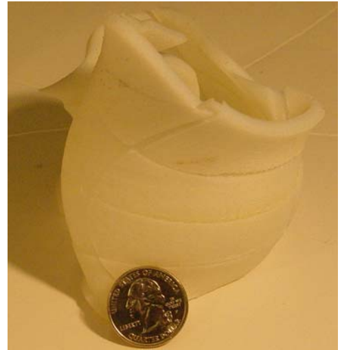
Figure 4.2 2" plastic model Model as small as 2" fabricated using Fusion Deposition Modeling (FDM)
