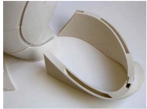
Figure 2.1 Interlocking components 3D fabricated models of interlocking assemblies
