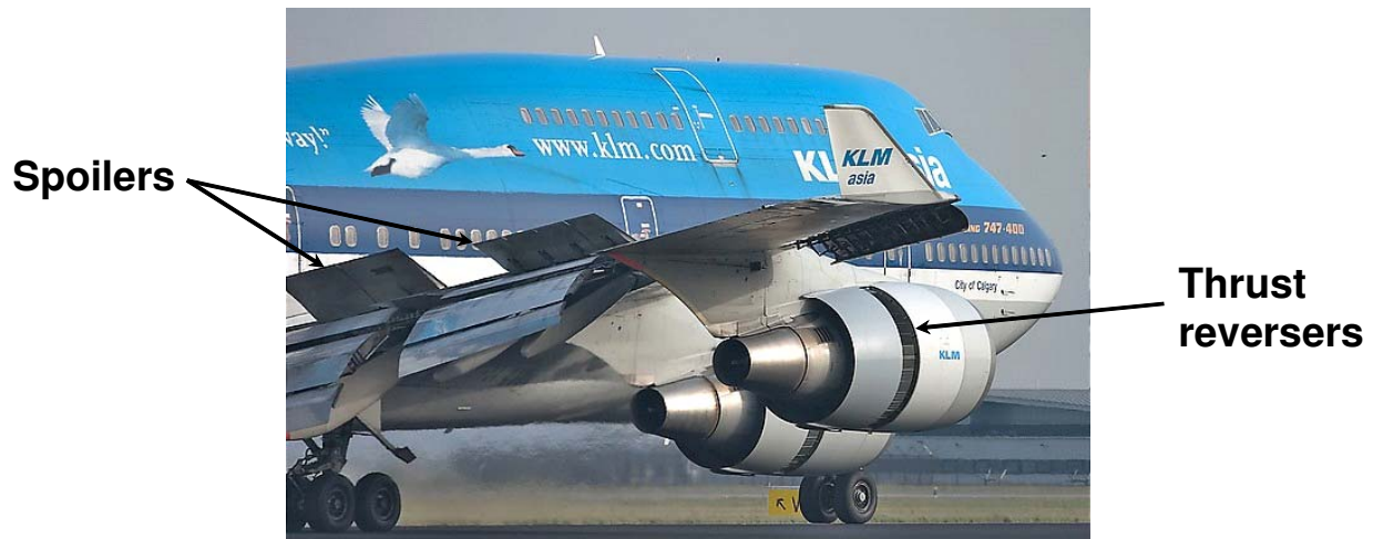
Figure 16: Thrust Reverser & Ground Spoilers Deployment [photo courtesy Marinus Bergsma]
