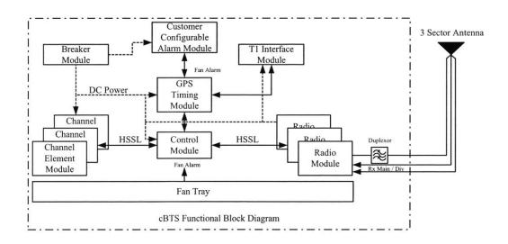
Figure 38 - CDMA cBTS High Level Functional Block Diagram
