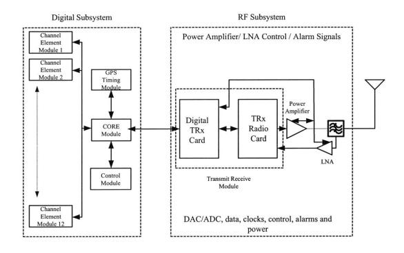
Figure 21 - DTRx Signal Flow within CDMA/UMTS BTS
