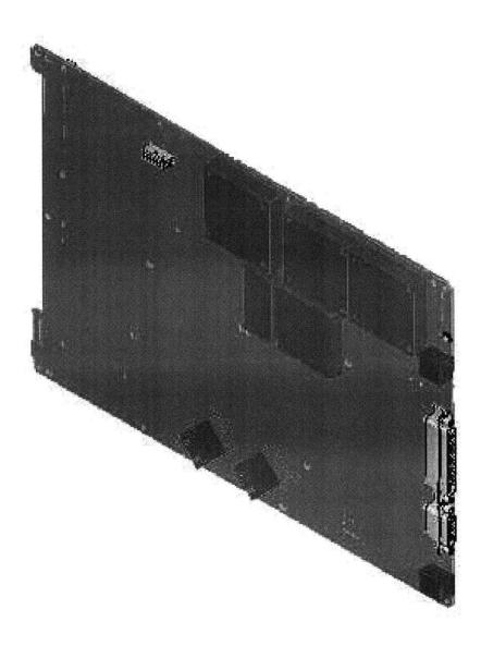
Figure 20 - DTRx Printed Circuit Card Assembly (FR-4) Physical Realization
