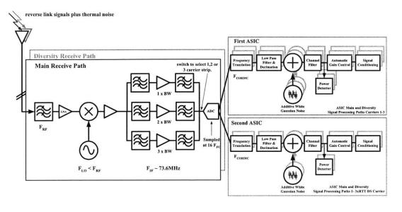
Main and Diversity RF and IF chains are located on the radio pcb
