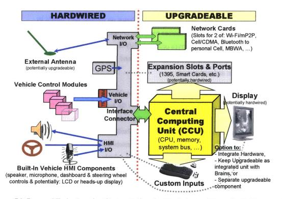
Figure 7.2: Proposed Technology Architecture Delineating Hardwired and Upgradeable Components
