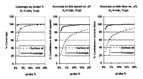
Figure 4.3: Geographic coverage & accuracy of traffic probe data versus percentage market penetration. For freeways, performance is greater than 95% above 3% penetration. [Dai et al]<sup>50</sup>
