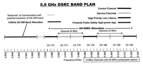
Figure 2.10: DSRC Band Allocation Plant (unratified)
