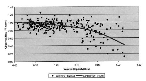
Figure 6.3: Observed Speed, as Percentage of Free-Flow Speed vs. Volume, as Percentage of Maximum Road Capacity for Highways in the Atlanta Metropolitan Area<sup>67</sup>
