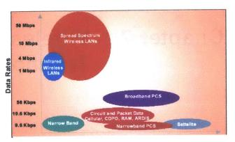
Figure 2.1: Wireless technologies data rate vs. coverage area or range.
