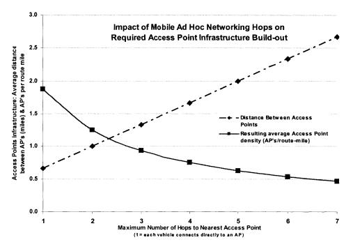
Figure 6.1: Access point density versus maximum number of mP2P hops
