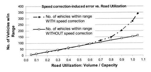
Figure 6.4: Speed Correction-Induced Error vs. Road Utilization<sup>68</sup>
