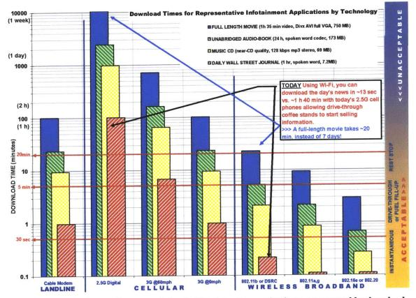
Figure 4.2: Application performance of bandwidth-intensive applications as measured by download times for six wireless and one wired technologies.
