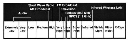
Figure 2.5: Wireless Radio Spectrum
