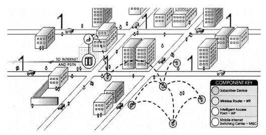
Figure 2.8: Illustration of mobile ad hoc system with connectivity to internet [MeshNetworks]
