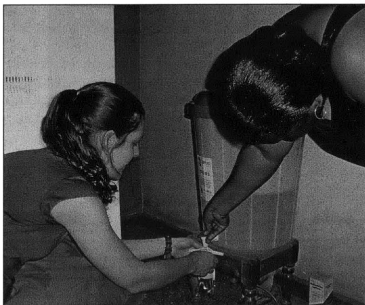
Figure 5: Water Sample Collection from the Tamakloe Filter Photo courtesy of Wahabu Salifu
