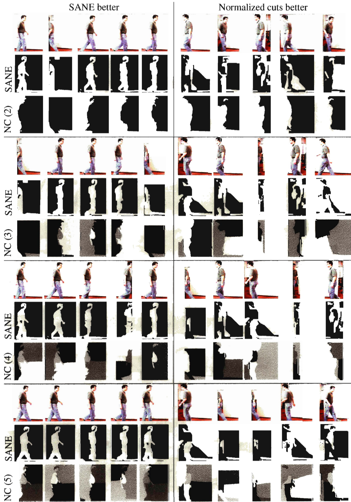
Figure 4-12: Walking examples in which SANE most outperformed Normalized Cuts, and vice-versa, for different numbers of Normalized Cuts regions.
