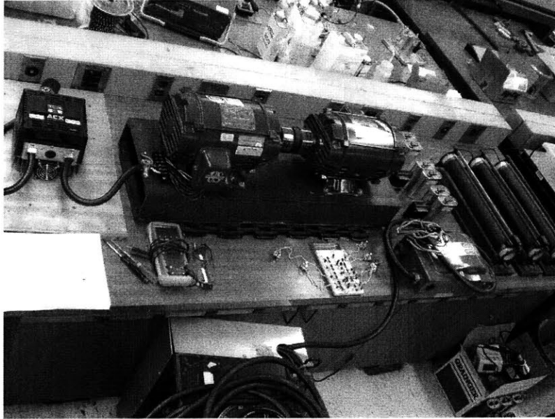
Figure 2.1: 2kW Test and Demonstration Platform
