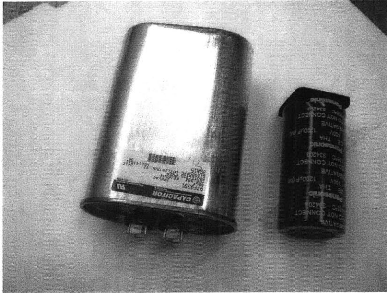
Figure 4.16: Comparison of 80 \mu\text{F} , 270 \text{ V} AC and 1200 \mu\text{F} , 400 \text{ V} DC capacitors
