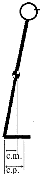
Figure 2.1. Human standing posture. c.m. : the center of mass, c.p.:the center of pressure
