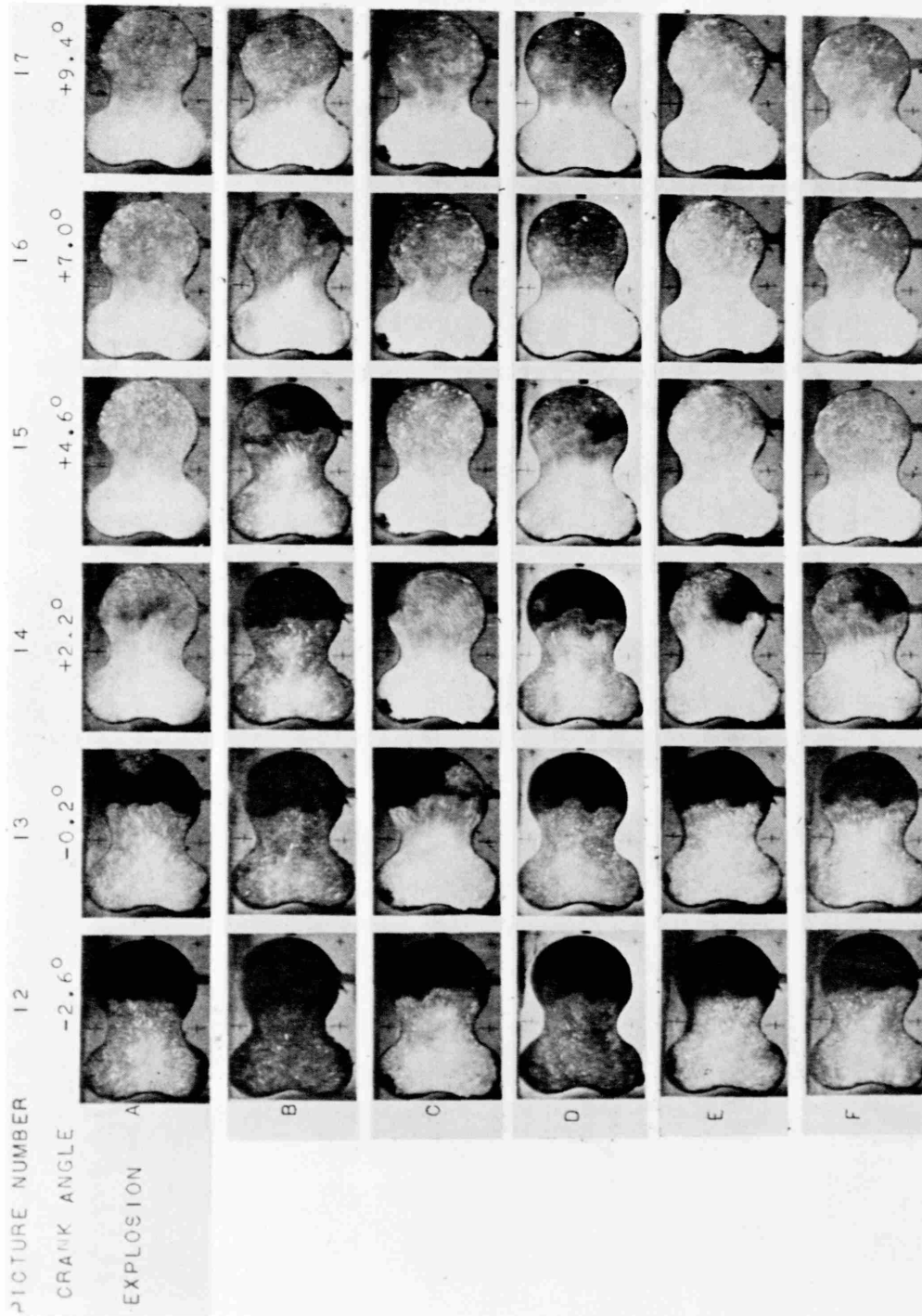
Occurrence of Knock in Six Different Explosions Photographed under Similar Engine Conditions REF. 154
