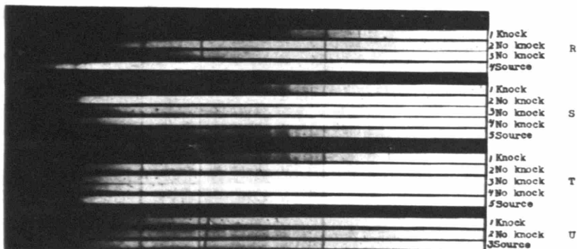
COMPARISON OF ABSORPTION BY CHARGES JUST PRIOR TO INFLAMMATION UNDER KNOCKING AND NONKNOCKING CONDITIONS WITH FUEL-AIR MIXTURE HEATED BEFORE ENTERING ENGINE
