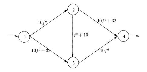
Figure 5-1: A generalized Braess' Paradox for which no link can be deleted.
