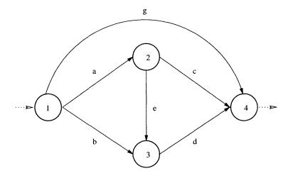
Figure 4-1: A network that violates the monotonicity of flow rates and the monotonicity of link loads.
