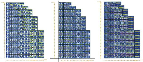
16-bit Domino CLA Adder 16-bit LSDL CLA Adder 16-bit Static CLA Adder Fig. 3.4. Adder layouts, by circuit architecture.
