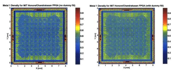
Fig. 2.12. Pattern density (with and without dummy fill) for MIT FPGA.
