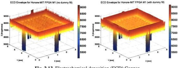
Fig. 2.13. Electrochemical deposition (ECD) Copper damascene envelope profile for MIT Honore/Chandrakasan Low Power FPGA. Without dummy fill (left) and with (right).
