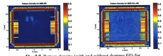
Fig. 2.8. Pattern density (with and without dummy fill) for BEE-generated layout.
