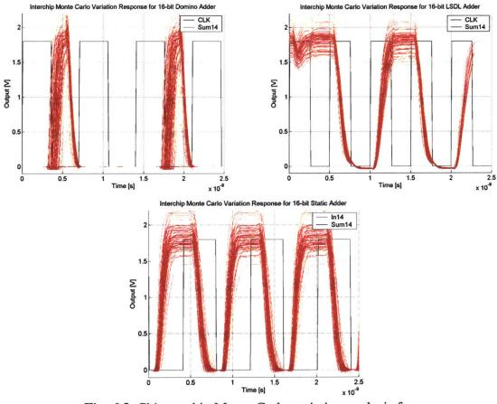
Fig. 6.3. Chip-to-chip Monte Carlo variation analysis for adder architectures.
