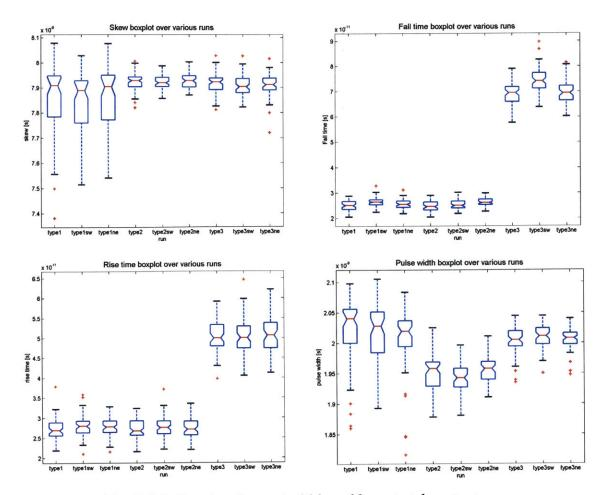
Fig. 7.6.2. Boxplots for centroid-based layout style output metrics. Grouped into types (1 = very regular, 2 = regular, 3 = non-regular). Among types, tests without slanted plane, with slanted plane into SW direction, and also into NE direction. In order from uppermost left to bottommost right: skew, fall time, rise time, and pulse width.
