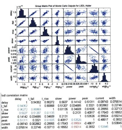
Fig. 6.9. Group plot matrix (above) and correlation matrix (below) for LSDL adder.
