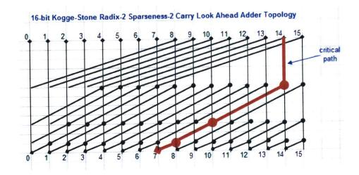
Fig. 3.3. Topology for 16-bit CLA adder design. Critical path is measured at SUM14.
