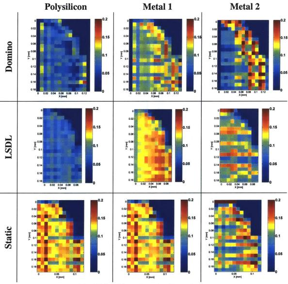
Fig. 5.12. Adder pattern density analysis.
