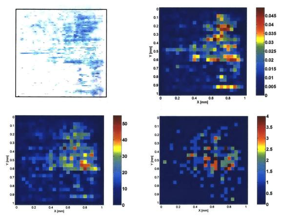
Fig. 2.6. Process binning for VPGA FPU Metal 1 interconnect. Metal 1 interconnect layout (upper left); Metal 1 interconnect pattern density (upper right); Bin 1 [0-0.35 μm] (lower left); Bin 2 [0.35-0.50 μm] (lower right).
