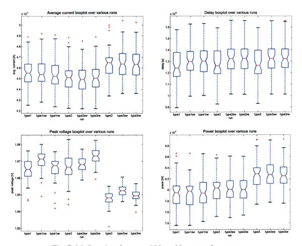
Fig. 7.6.1. Boxplots for centroid-based layout style output metrics. Grouped into types (1 = very regular, 2 = regular, 3 = non-regular). Among types, tests without slanted plane, with slanted plane into SW direction, and also into NE direction. In order from uppermost left to bottommost right: current, delay, peak voltage, and power.
