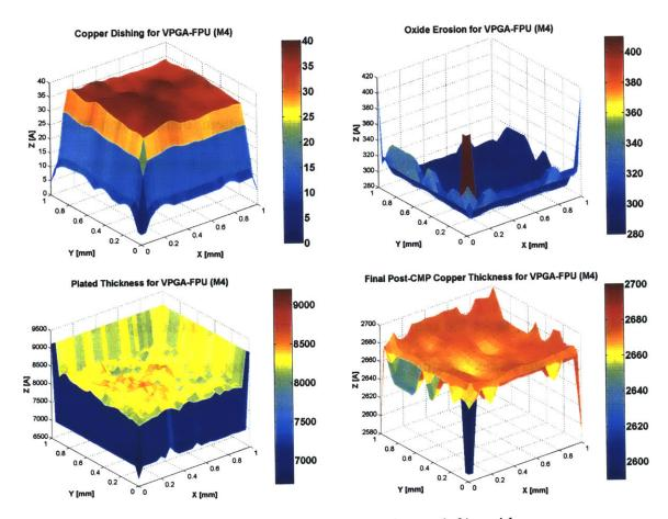
Fig. 2.7. Modeled copper thickness (upper left), oxide erosion (upper right), plated thickness (lower left), and post-CMP copper thickness (lower right) for VPGA FPU's metal 4 interconnect.
