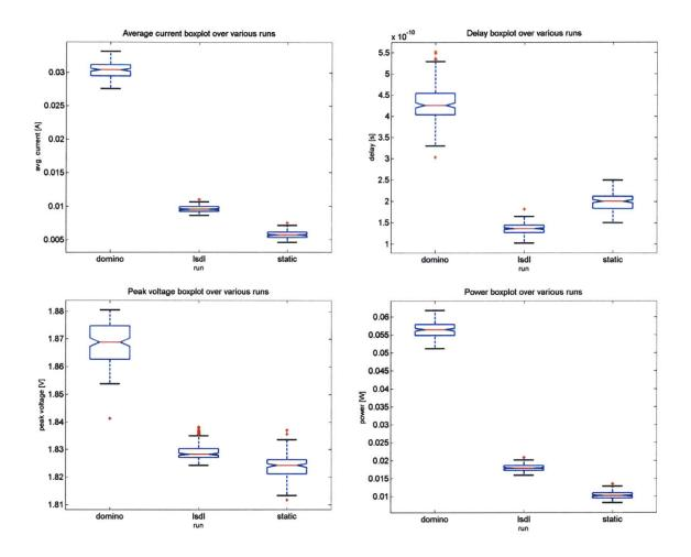
Fig. 6.7.1. Boxplots for adder output metrics. In order from uppermost left to bottommost right: current, delay, peak voltage, and power.
