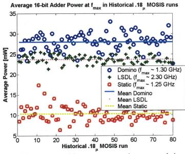
Fig. 4.2. Average adder power at maximum speeds in historical MOSIS process models.
