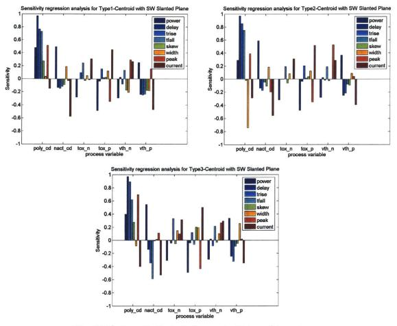
Fig. 7.7.3. Sensitivity tests for centroid-based inverter chain layouts, with southwest slanted plane. Type 1-very regular (upper left), type 2-regular (upper right), and type 3-non-regular (bottom).
