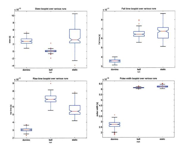
Fig. 6.7.2. Boxplots for adder output metrics. In order from uppermost left to bottommost right: skew, fall time, rise time, and pulse width.
