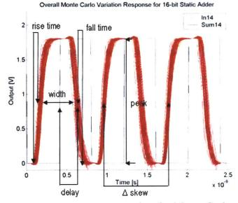
Fig. 6.5. Output measurements taken for Monte Carlo runs.
