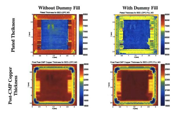
**Fig. 2.10.** Plated thickness and post-CMP copper thickness (with and without dummy fill) for BEE-generated layout.
