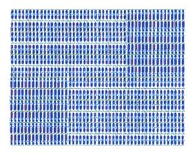
Fig. 7.5. Layout of very regular inverter chain, with grouped cells and matching centroids among blocks.
