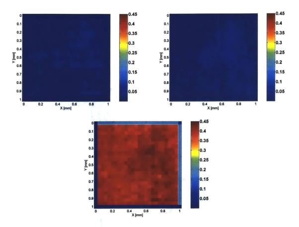
**Fig. 2.5.** Normalized VPGA Metal Densities. Metal 1 (upper left); Metal 2 (upper right); Metal 3 (lower).
