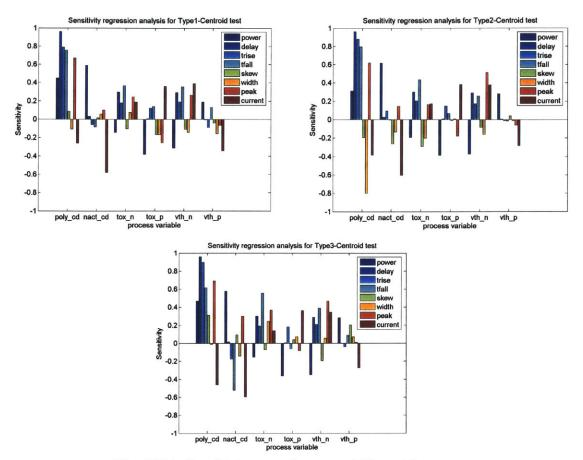
Fig. 7.7.1. Sensitivity tests for centroid-based inverter chain layouts, with no slanted plane. Type 1-very regular (upper left), type 2-regular (upper right), and type 3-non-regular (bottom).
