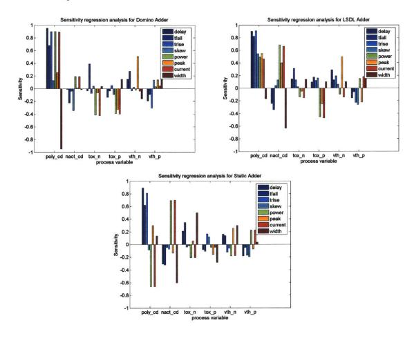
**Fig. 6.6.** Multiple regression sensitivity analysis for Monte Carlo adder simulations. Domino adder (upper left), LSDL adder (upper right), static adder (bottom).
