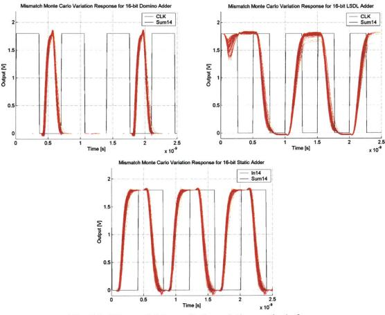
Fig. 6.2. Mismatch Monte Carlo variation analysis for adder architectures.
