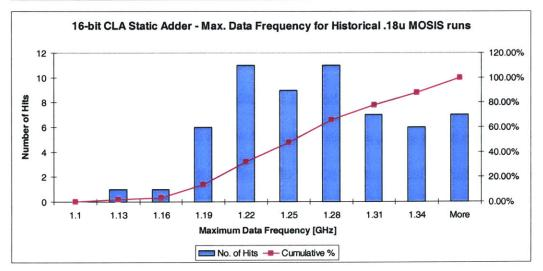
Fig. 4.1. Maximum adder speeds and distributions under historical MOSIS process models.
