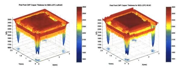
Fig. 2.11. 3D visualization of BEE-generated decoder metal 3 layer, post-CMP. Without dummy fill (left) and with (right).
