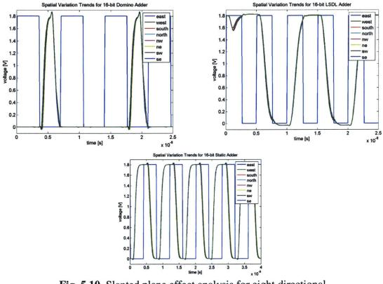
Fig. 5.10. Slanted plane effect analysis for eight directional trends (strength into direction).
