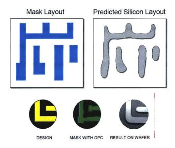
Fig. 1.2. Increasing geometrical primitives increases uncertainty in final design [1].
