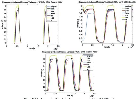
Fig. 5.11. Impact of isolated process variable (110% of nominal value) on adder performance. Domino adder (upper left), LSDL adder (upper right), static adder (bottom).
