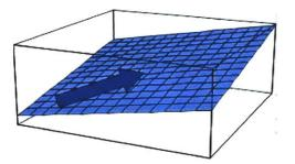
Fig. 7.1. Suggested linear process variation gradient (slanted plane effect).
