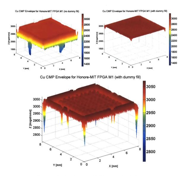
Fig. 2.14. 3D Visualization of MIT Honore/Chandrakasan low power FPGA, post-CMP. Without dummy fill (upper left) and with (upper right). Zoom of profile with dummy fill (bottom).
