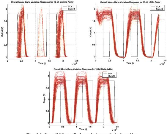
Fig. 6.4. Overall Monte Carlo variation analysis for adder architectures.
