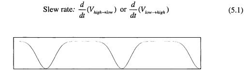
Fig. 5.5. Non-desirable clock slew.
