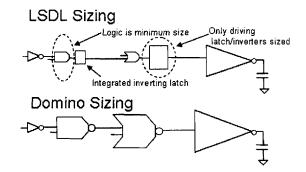
Fig. 3.2. LSDL sizing vs. domino sizing.
