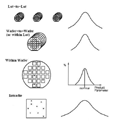
Fig. 2.2. Scope of variation in semiconductor manufacturing [6].
