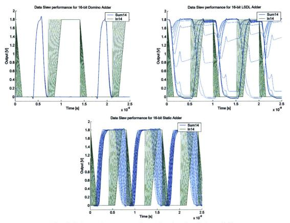
Fig. 5.7. Data slew comparisons for domino (upper left), LSDL (upper right), and static (bottom) adders.
