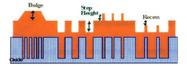
Fig. 1.4.1. Copper plating problems due to irregular pattern density in design [2].
