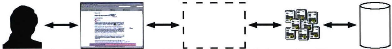
Figure 3-15. The Webbed Footnotes system architecture. From left to right: the user, the web browser (containing the Webbed Footnotes extension), the hidden browser frame, several PHP scripts residing on the web server, and the SQL database.
