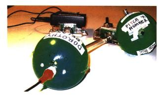
Figure 5: Microphone with Variable Delay
