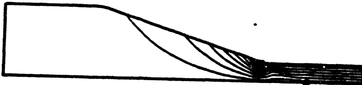
Figure 6.21k Contour plots of \text{Det}_{\tau_{rz}} in the flow through a 4:1 conical contraction with rounded corners for N=4.0 , \sigma=1.0 , \beta=1.6 \times 10^{-5} and De=0.1 , 1.0 and 5.0.
