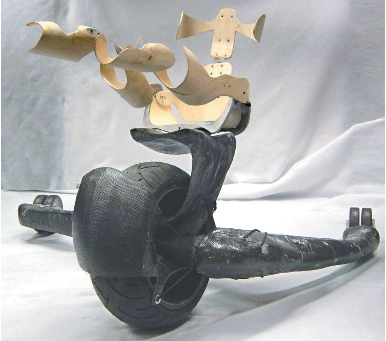
Finalized model. Carbon frame and wheel, plywood seat, muscle tendons piercing through the arm to control the wheel. Design overall: Axel Kilian. Robotic wheel and arm: Peter Schmitt, Axel Kilian Humane Seat: Patrik Künzler, Enrique L. Garcia, Axel Kilian.
