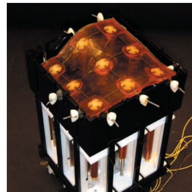
Computer numerically controlled pistons drive the surface into the desired position.
