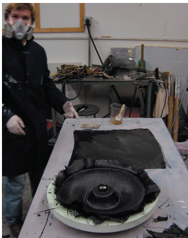
Fabrication of the full scale design in carbon fiber based on molds in mdf and soft foam plugs. All molds and plugs were CNC milled. Rim mold shown by Peter Schmitt.
