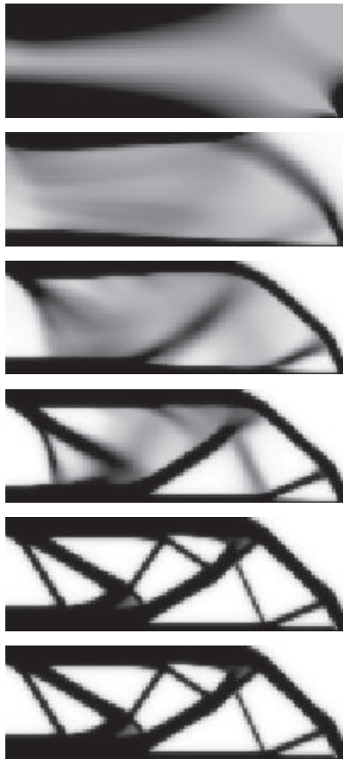
Sequence of a truss topology optimization over time from a set of forces. in two dimensions. (top)
