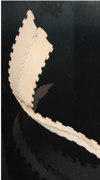
An aluminum assembly with pressure fit rubber strip. Early waterjet aluminum cut model 1999..
