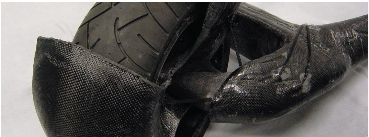
Finalized model. Carbon frame and wheel, plywood seat, muscle tendons piercing through the arm to control the wheel. Design overall: Axel Kilian. Robotic wheel and arm: Peter Schmitt, Axel Kilian Humane Seat: Patrik Künzler, Enrique L. Garcia, Axel Kilian.
