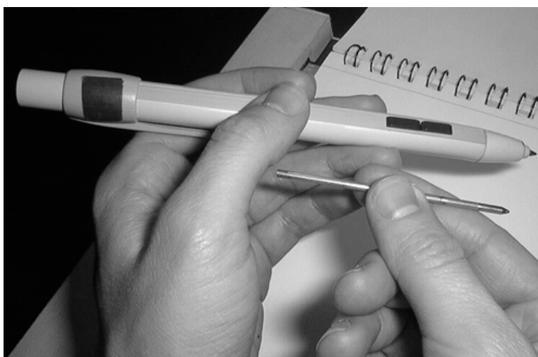
Figure 3-3: Notes are taken with a digitizing pen equipped with an ink cartridge.
