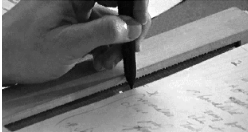
Figure 3-32: In this photo, the user fine-tunes the starting point of playback using the audio cursor and scrollbar.
