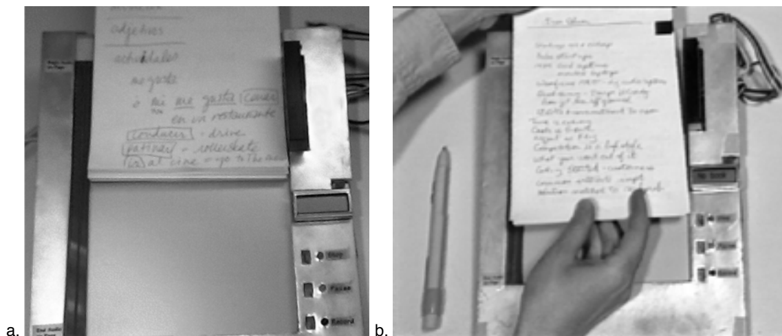
Figure 3-9: The user slides (a) or places (b) a notepad into the device (version 1 prototype).
