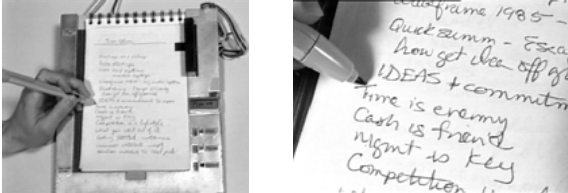
Figure 3-11: The user can randomly access different parts of the audio recording by pointing to a location in his/her notes (version 1 prototype).
