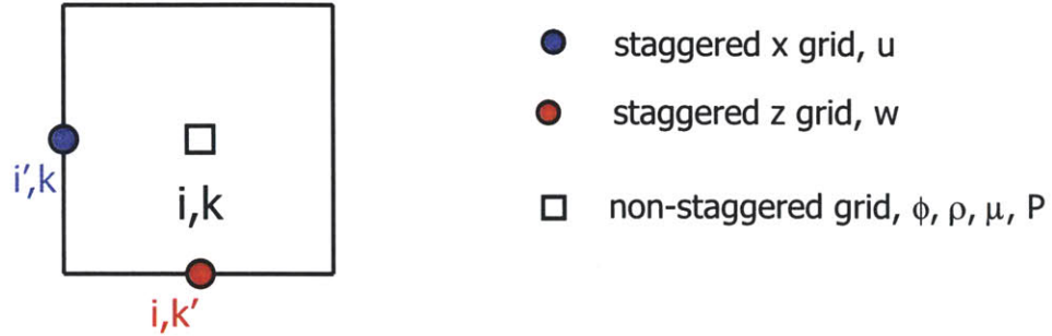
Figure 3-1: Schematic of the MAC-type grid used in the discretization of the level set formulation.
