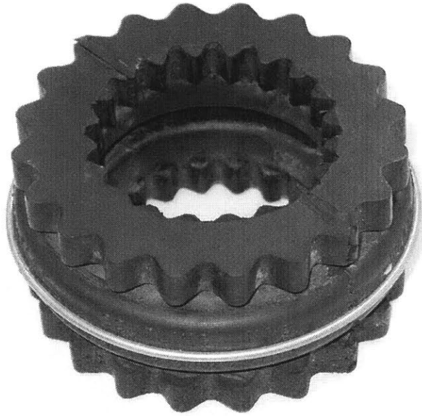
Figure 5.12: ASW Pump Motor-to-Impeller Coupling
