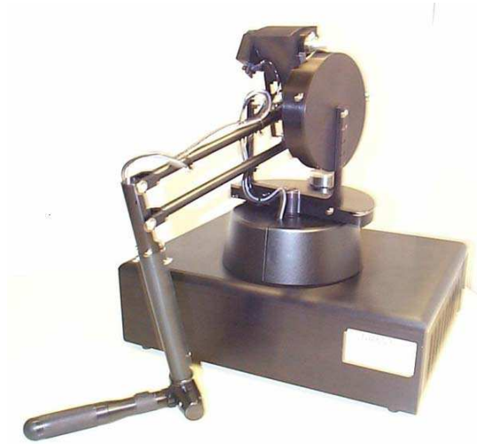
Figure 5-1: PHANTOM haptic device
