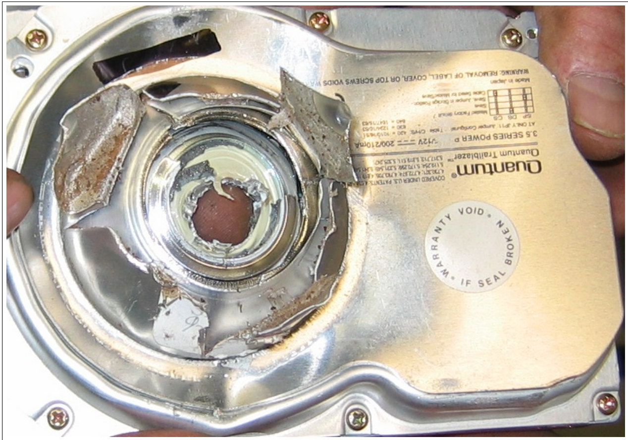
Figure 3-4: A hard drive that was punched with a new machine that is being developed by Charles Smith of Greenville SC as a result of having read [GS02a]. Although this approach is easy to audit, it is probably not sufficient for classified material. Photo used with permission.
