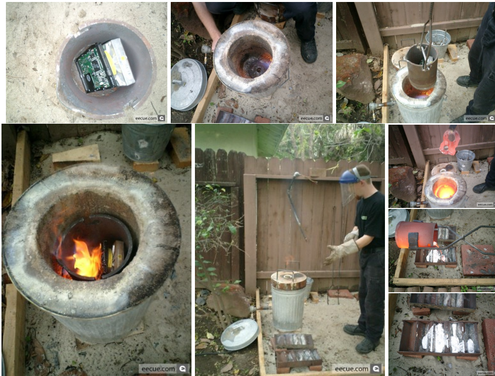
Figure 3-3: Drive Slagging Following the publication of [GS02a], Dave Bullock, John Norman and “CHS” performed this demonstration of melting a hard disk with gas-fired furnace that they had built in a back yard. The authors concluded: “Drive slagging is a fool-proof method to prevent data recovery.” Photos used with permission.
