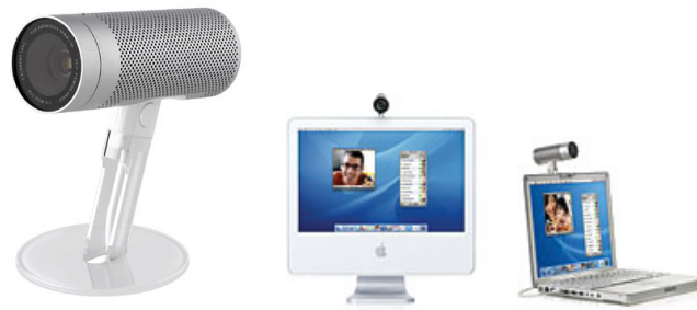
Figure 9-1: Apple's iSight camera is designed to sit atop a computer screen and point directly at the user. The camera includes a built-in microphone.
