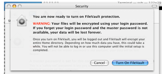
Figure 2-24: When File Vault is first enabled, it creates a cryptographically protected virtual disk, copies the user’s files to that disk, and then deletes unencrypted files. Analysis of a disk revealed that File Vault does not use Complete Delete to delete the unencrypted files. As a result, they can be recovered using forensic tools.
