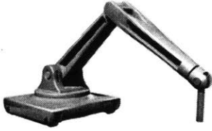
Figure 92 - An early version of the pick-and-place machine with 3-Link connection
