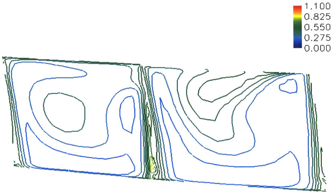
Figure 4.17a - Mass 2 - Entropy generation contour at enhanced impeller exit - t=t_0
