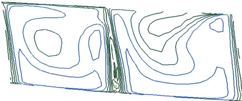
Figure 4.17c - Mass 2 - Entropy generation contour at enhanced impeller exit - t=0.8T
