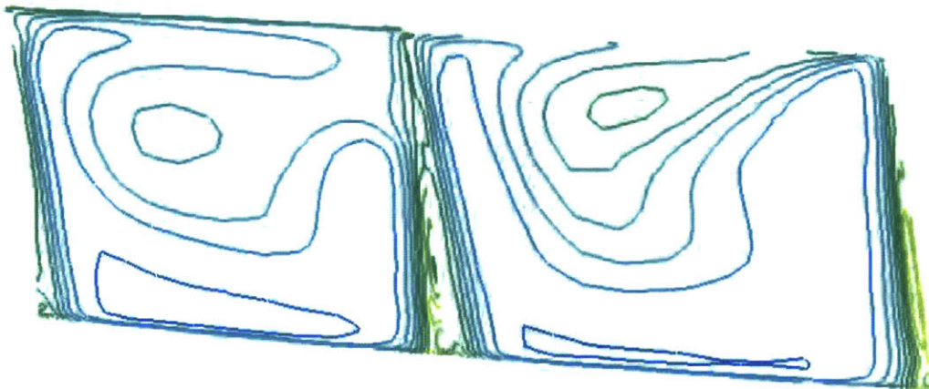
Figure 4.15b – Mass 1 - Entropy generation contour at enhanced impeller exit – t=0.4T
