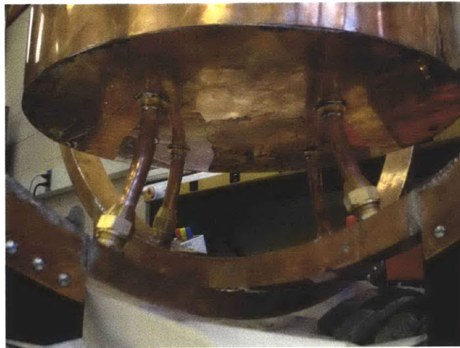
Figure 3.14: Tank Connection Pipes
