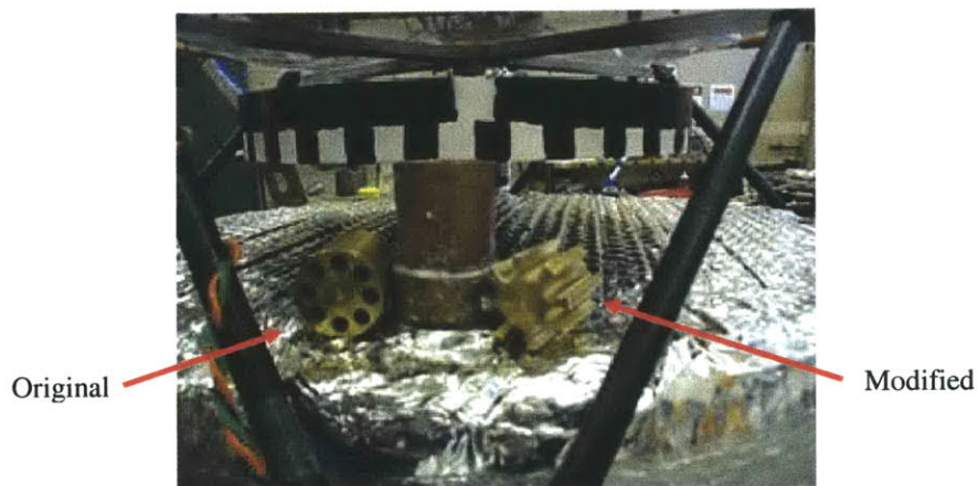
Figure 3.19: Pressure Regulator Fix
