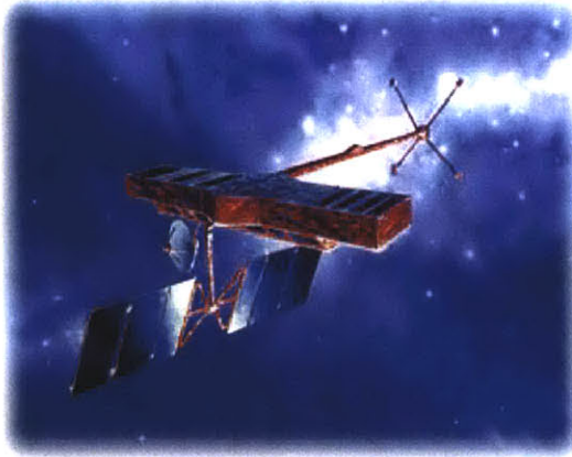
Figure 1-1: Space Interferometry Mission (SIM), one of the projects of the Origins Program by NASA, is a space observatory aimed at determining the positions and distances of stars several hundred times more accurately than any previous programs. It is planned to launch in 2009.
