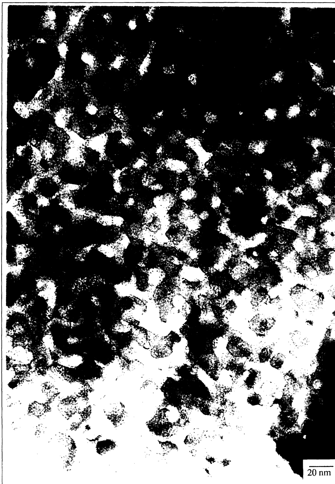
Figure 5.5b Plan view TEM of a LaAlO 3 film derived from lanthanum-aluminum nitrates (at lower magnification).
