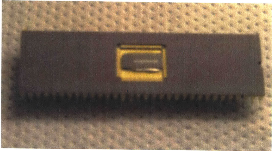
Figure 3-4: Image of the packaged optical MEMS switches evaluated in the Zygo profilometer system.
