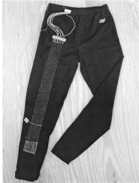
Figure 4-1 Spandex pants with conductive fiber sensors for lower body monitoring
