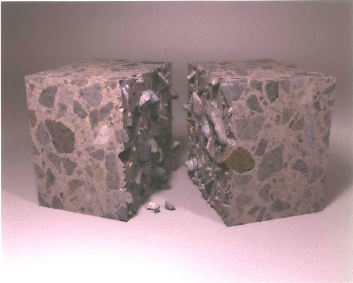
Figure 7-5: A synthetic image of a concrete box is created by splitting the geometry with a simple plane while respecting particle shape boundaries. This demonstrates an advantage of having an explicit spatial texture representation
