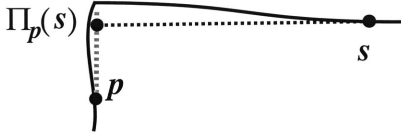
Figure 4-3: When \mathbf{s} and \mathbf{p} are on opposite sides of the corner and Jones et al.'s [2003] predictor is used, the distance between \Pi_{\mathbf{p}}(\mathbf{s}) and \mathbf{s} depends mostly on \mathbf{s} 's distance from the corner.
