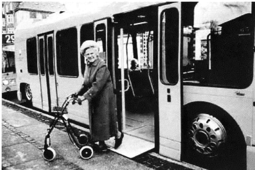
Figure A9: Improved accessibility with low-floor axles
