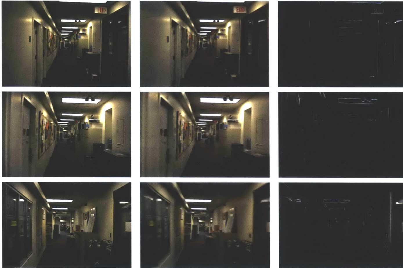
Figure 5-11: A comparison of original images (first column) to rendered images (second column). The third column shows the absolute value of differences between the images in the first two columns.
