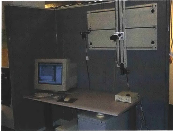
Figure 1-6: MIT's single-camera light field capture device.
