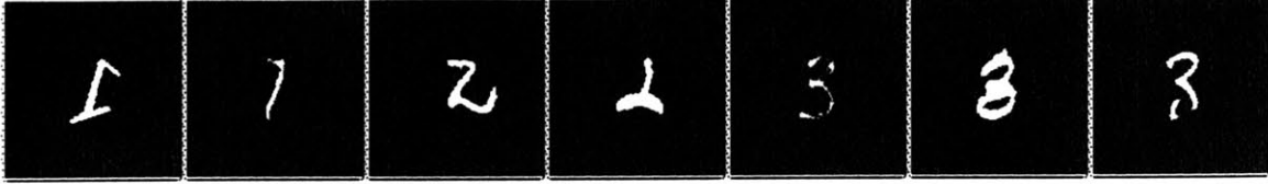
Figure 5-7: Difficult cases that congealing handled well. These are the images after congealing has aligned them to the model as well as possible. The first two cases are “1”s with unusual or spurious strokes. The third frame shows a “2” with an unusual tail. The algorithm essentially ignored the tail and aligned the rest of the character. The fourth frame shows a “2” that has been clipped, but the algorithm puts the remainder of the character in correspondence with the model. The last three cases are all “3”s, with missing pixels, spurious stroke, and clipped bottom respectively.
